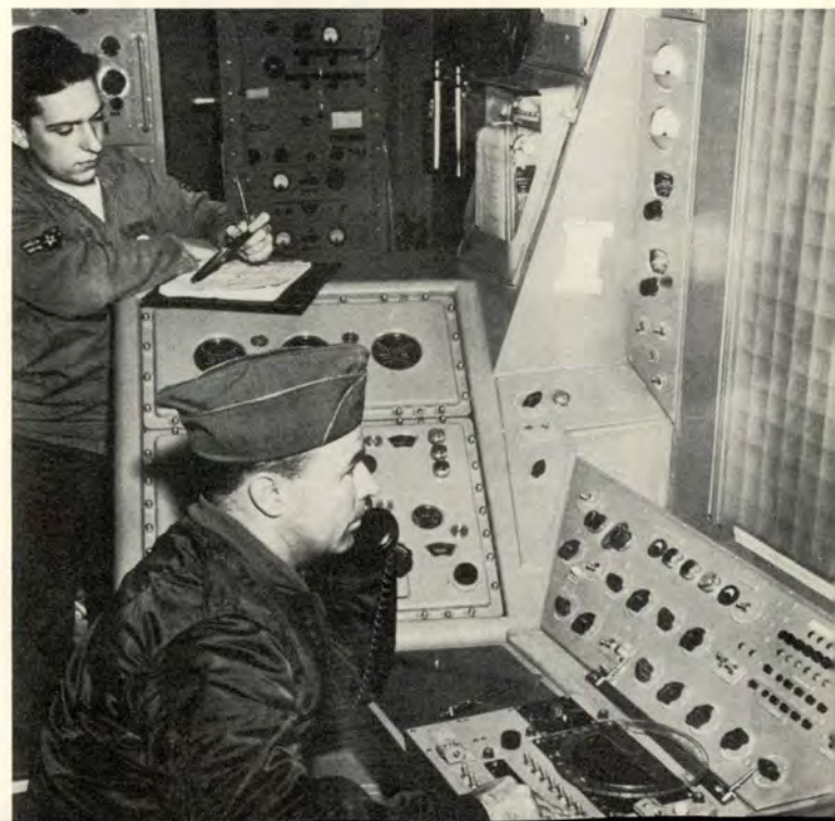
A runway controller flies the QF-80 off the runway, then a DT-33 director aircraft controls it to the orbit area, and a ground radar controller directs the pilotless aircraft through the atomic cloud.
