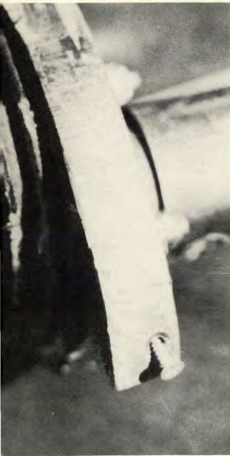
Left, shows how the bolt backed off of lock nut. Below, cover plate removed exposes the critical area where loose bolt caused the jammed control.
