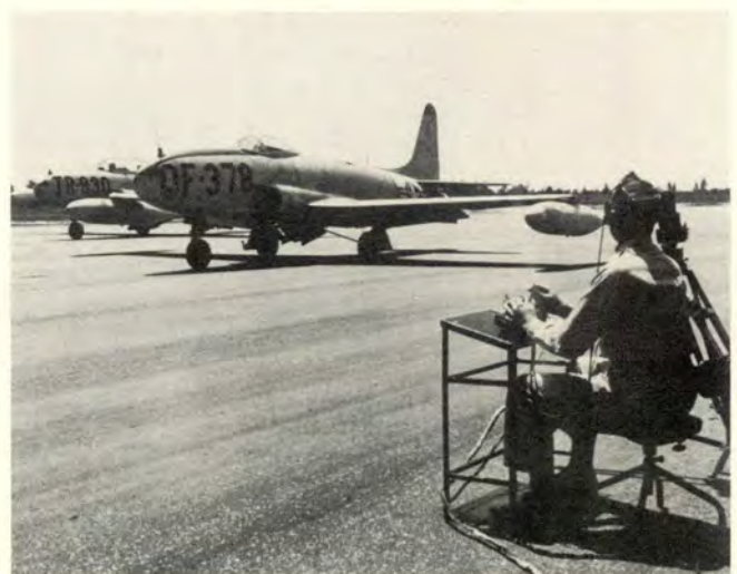
A runway controller flies the QF-80 off the runway, then a DT-33 director aircraft controls it to the orbit area, and a ground radar controller directs the pilotless aircraft through the atomic cloud.
