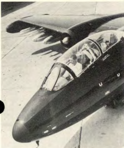
The underslung design of the aircraft creates an illusion of taxiing in a nose-low attitude.
