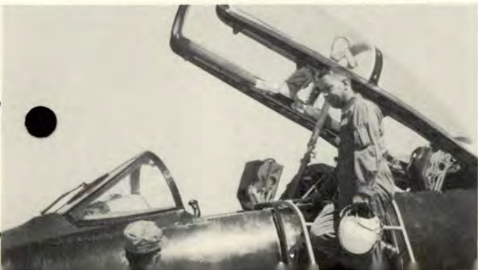
The single, bubble canopy is hinged at the rear to afford easy entry.
