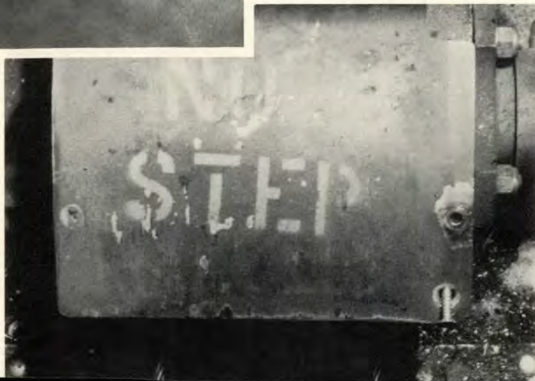
Left, shows how the bolt backed off of lock nut. Below, cover plate removed exposes the critical area where loose bolt caused the jammed control.
