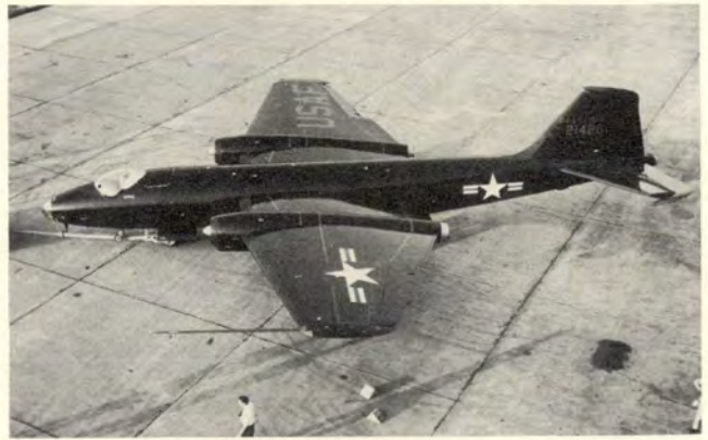
The RB-57 has a smaller canopy that covers the pilot's cockpit only.
