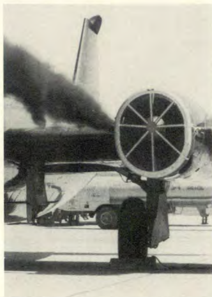
During starting operations, black smoke from the cartridge escapes from the engine exhaust port.
