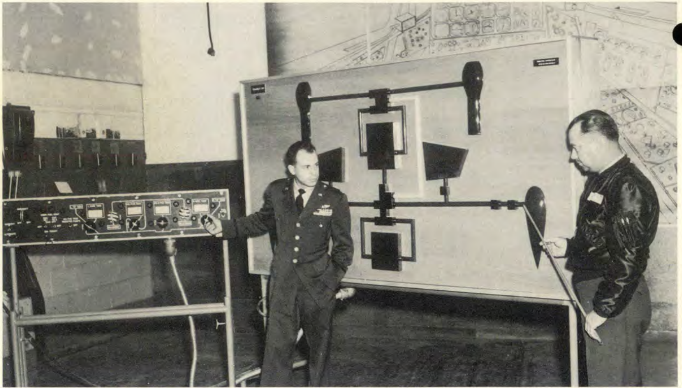
A ground school training aid shows fuel-flow control panel arranged in a schematic flow pattern so that overall operation can be seen at a glance.
