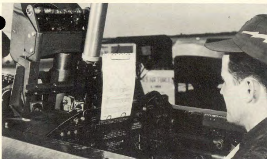
A holder for the jet letdown chart, improvised from a coat hanger, fitted on the panel of a T-33.
